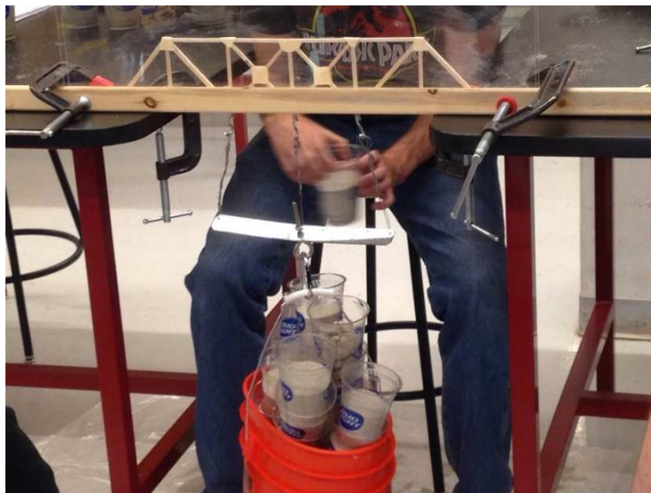
Figure 5. Truss bridge design project testing setup
