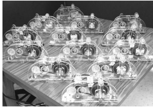
Figure 3. A full complement of Haptic Paddles to outfit a mechatronics lab has been manufactured and assembled.
