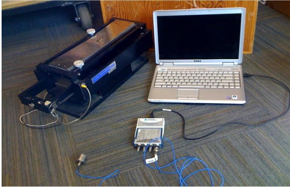
Figure 1: Test equipment (shaker, accelerometer, DAQ, computer).
