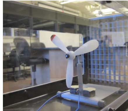
Figure 5. Turbine cart for wind tunnel
