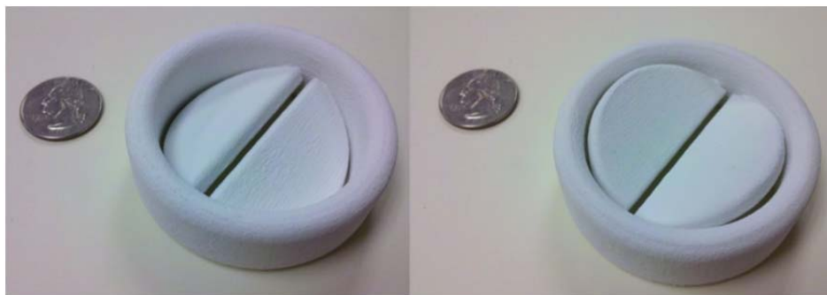
Figure 5: Traditional Bi-leaflet SMK2 Mitral Valve 1:3 Scale Printed out of Starch Front and Back Views
