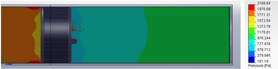
Figure 8: SMK1 Mitral Valve at 90° Pressure Flow Simulation
