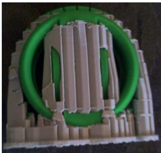
Figure 6: SMK2 Mitral Valve in ABS Plastic shown with subset
