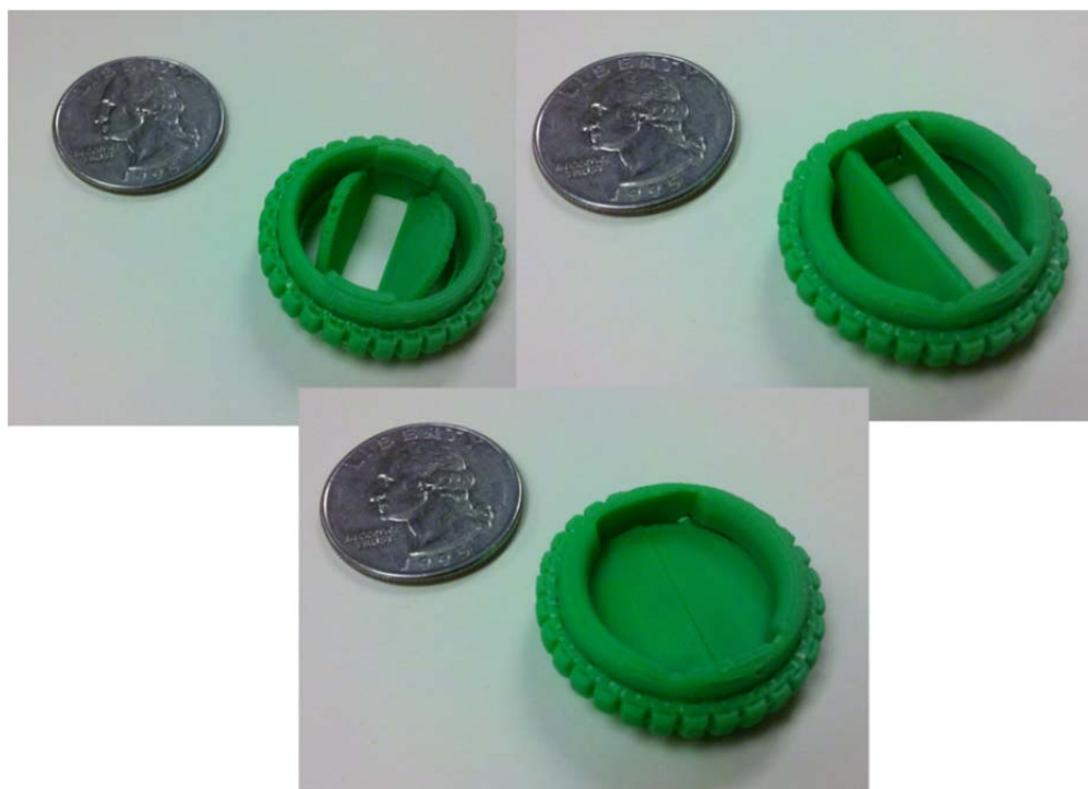
Figure 7: SMK2 Mitral Valve Assembly with Suture Ring in ABS Plastic 1:1 Scale Top, Bottom and Closed View
