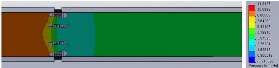
Figure 10: SMK2 Mitral Valve at 85° Pressure Flow Simulation
