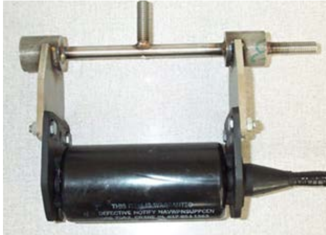
Figure 4. Original Hydrophone in Existing Mounts
