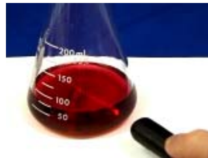
Figure 4. A reddish suspension of gold nanoparticles is produced by reduction of a gold (III) salt. The presence of the gold colloid can be detected by the scattering of a laser beam by the nanoparticles. 29
