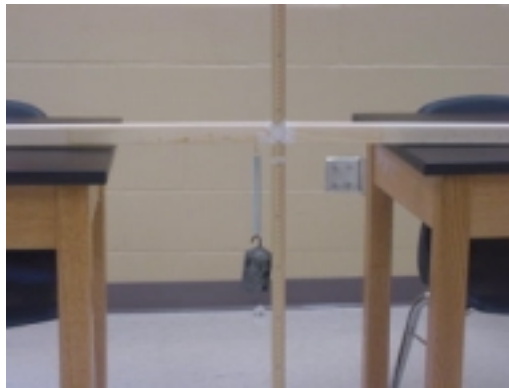
Figure 3: Illustration of setup for Hooke's Law activity
