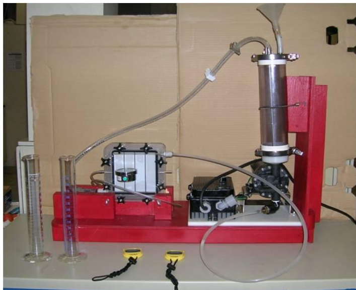
Figure 3. Photograph of Experimental Apparatus for BSA Protein Recovery
