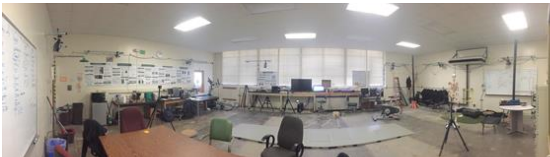
Figure 1. Panoramic Image of HMB Lab with near InfraRed cameras mounted on the walls to capture live motion.
