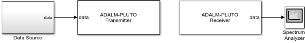
Figure 9. Communications System Toolbox for the PlutoSDR in Simulink.
