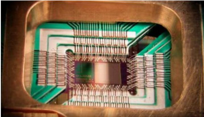
A close-up of a D-Wave One computer chip. (D-Wave Systems, Inc.)
