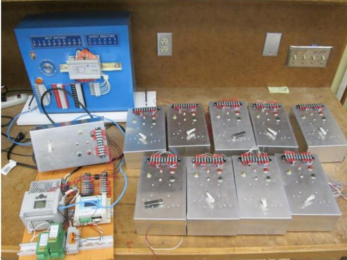
Figure 6 shows the in-house built Micrologix 1100 PLC board and Motor Control Boxes
