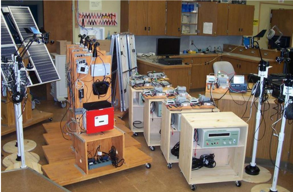
Figure 1 This picture shows some of the equipment developed in-house for alternative energy SCADA training. The large roller platform in the center housed an inverter and a weather station that was monitored wirelessly. On the side of the roller platform PLC training cards could be mounted for monitoring the inverter voltage and current and passing information to a SCADA system.
