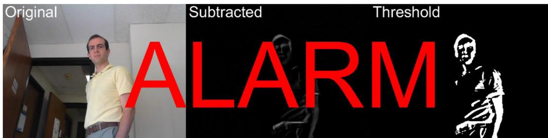
**Fig. 4:** MATLAB figure for motion detector. The original image converted to grayscale, subtracted from the previous image, then thresholded according to the sensitivity level. If a defined fraction of pixels are triggered, then the alarm is activated. Note that the author moved prior to the image shown. (Face covered with white box for review process only)
