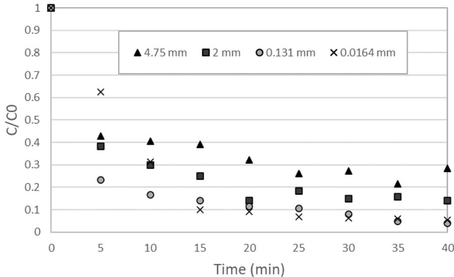
Figure 2. Changes to turbidity concentration, normalized to initial NTU, over time for varying sized granular media. Smaller grain-sizes correlated with faster turbidity removal and lower stabilized effluent turbidity, though head loss was severe.
