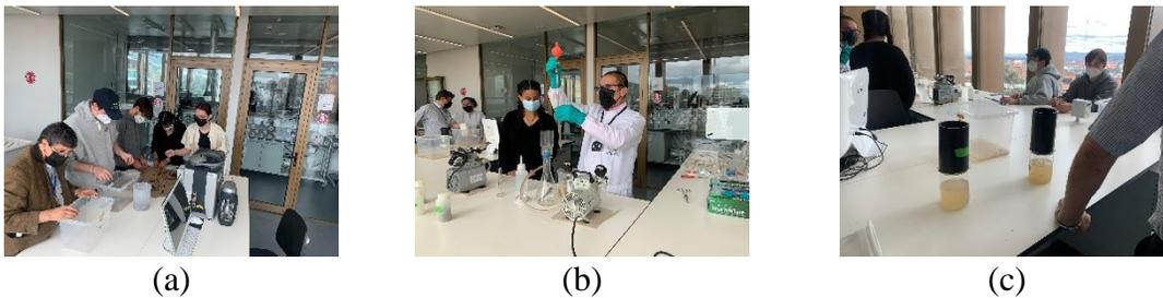
Figure 3. Experimental Testing as Pontificia Universidad Javeriana Bogotá: (a) removing cherry coffee mucilage layer, (b) total suspended solids test, and (c) filtration tests.
