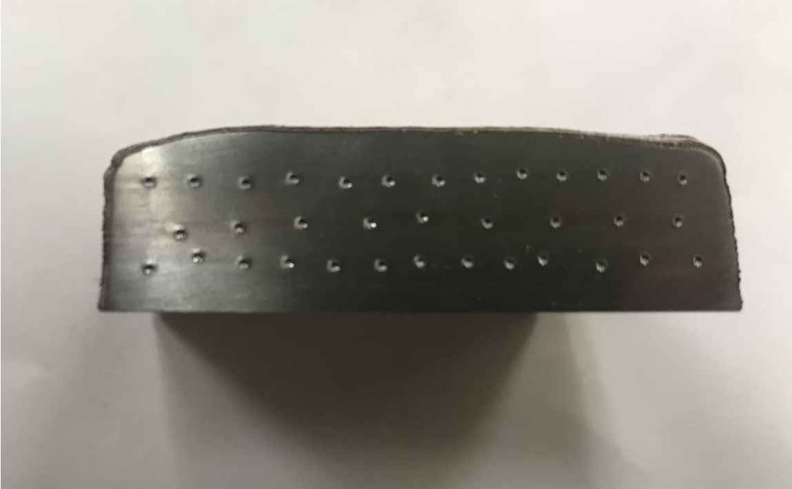
Figure 3: As-built Ti 64 sample showing the polished side and the Rockwell indents.
