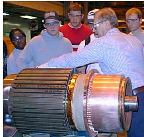
The students toured the factory where the motors are manufactured from the ground up. The copper windings are shaped and wrapped with insulation, and then inserted into the stator core. The students also saw where the rotor was machined and integrated with the commutator (for the dc motor). The students saw how the motors were both balanced for vibration and performance tested.
