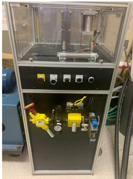
Fig. 7. Safety demo with pneumatic lockout and electronic control valve.
