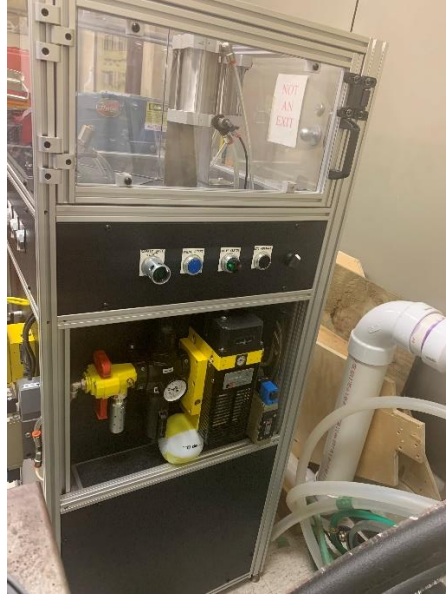
Fig. 8. Safety door latch and control valving.
