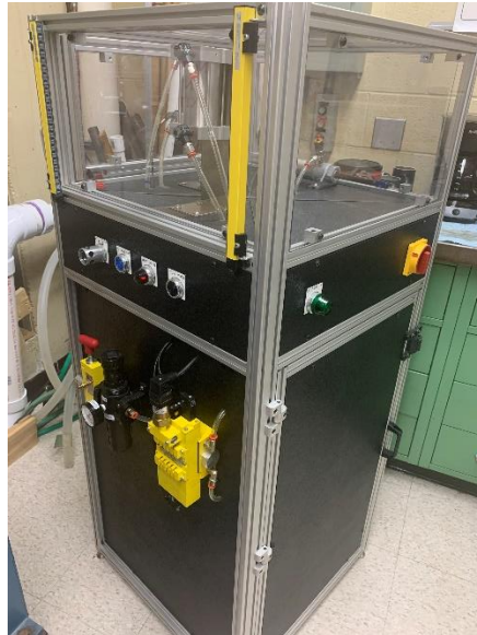
Fig. 9. Safety demo with light curtains and electronic control valving.
