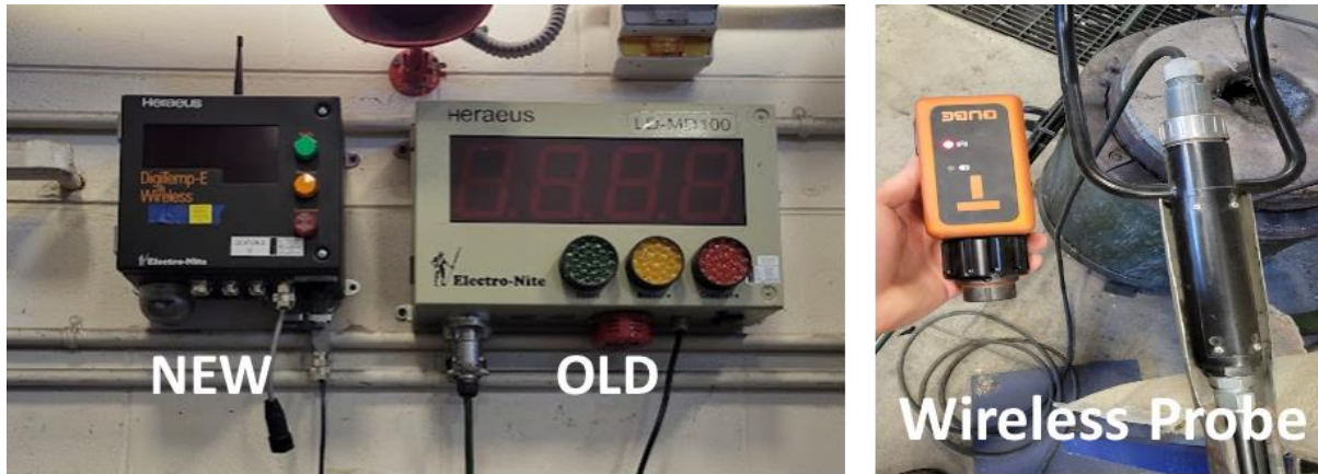
Fig. 2. Upgraded wireless temperature display module and wireless probe.
