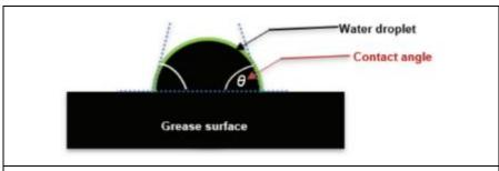
Figure 1. A Visual Representation of the Contact Angle Approach.
