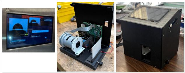
**Figure 2.** (*Left*) The contact angle as measured by the current prototype. (*Middle*) The internal components. (*Right*) The current assembled prototype of the Contact Angle Instrument by Koehler Instrument Company, Inc. and Farmingdale State College (FSC).
