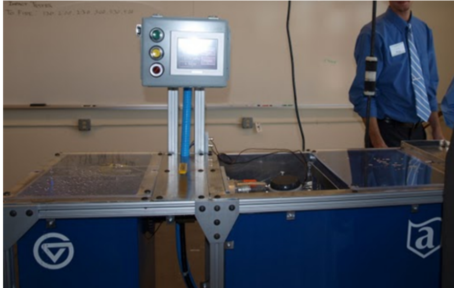
Figure 3 - The Test Stand with Touch Screen Interface
