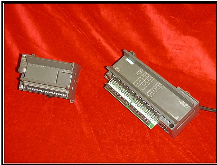
FIGURE 3 Siemens Micro Programmable Logic Controllers Used in ICS-1
