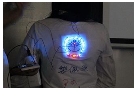
Fig. 2. Wearable optoelectronic design project in which a Doraemon image was outlined with blue and red LEDs operated in CW mode 9 .
