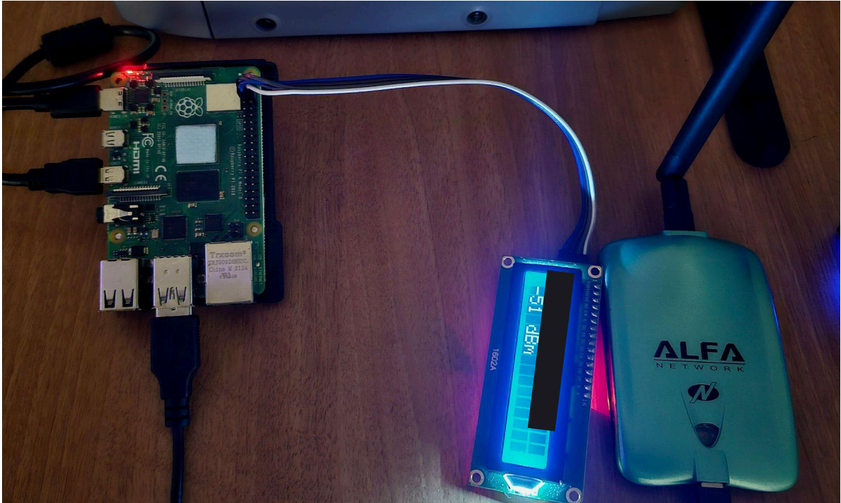
Figure 3 - Hardware for data collection displaying MAC and RSSI values
