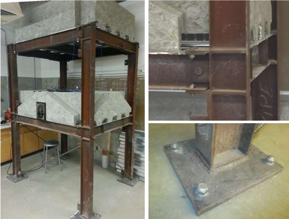
Figure. Two-story Steel Frame, Beam/Column Connection and Column Base Connection
