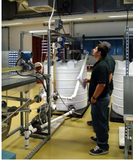
Figure 1: Students at a flow loop station. Pump, Coriolis and magnetic flow meters, and water reservoir visible.
