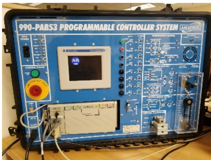
Figure 8. Amatrol PLC portable training station
