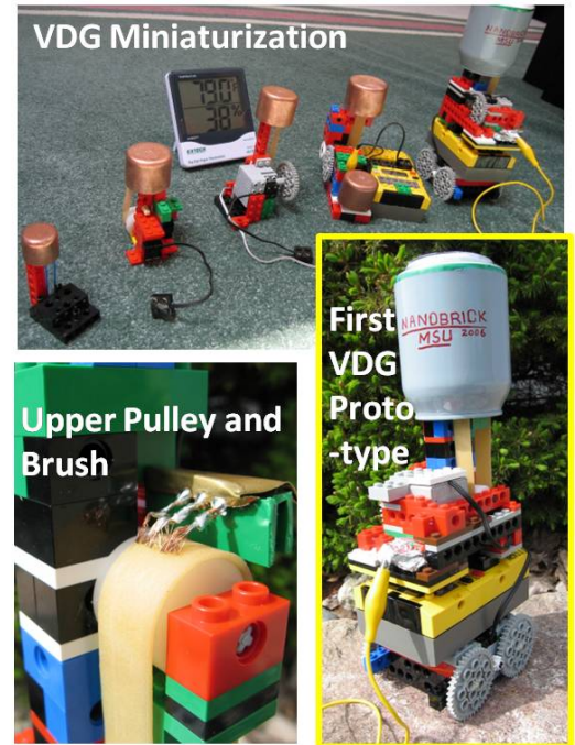
Fig. 2 Programmable robotic VDG generator; miniaturization of VDG and a close-up of upper pulley and brush.
