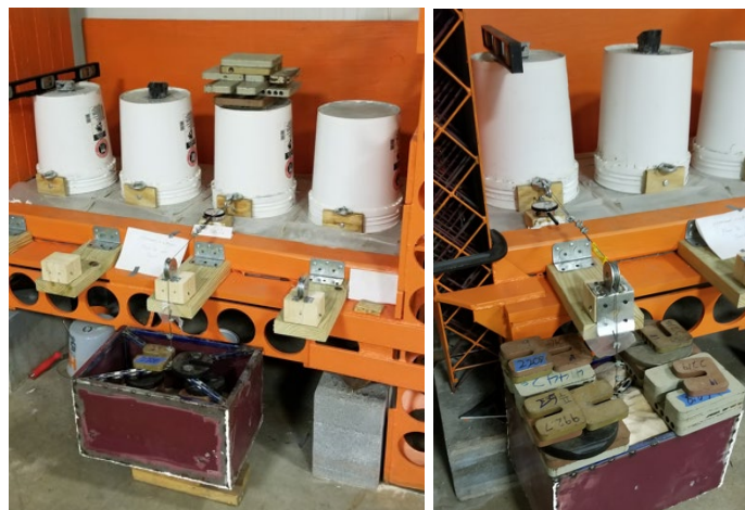
Figure 2- Concrete specimens under gradually applied loads.
