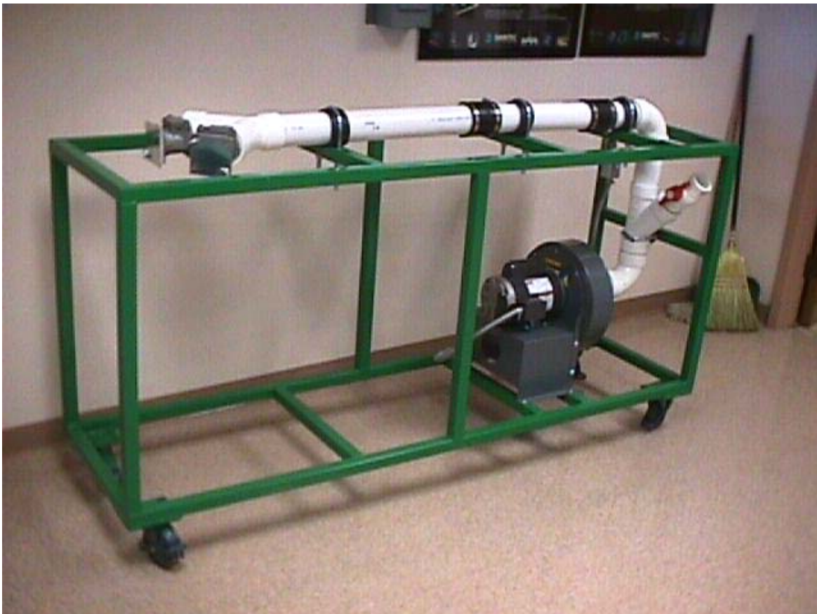
Figure 2. – MAFs, frame, and blower-motor assembly
