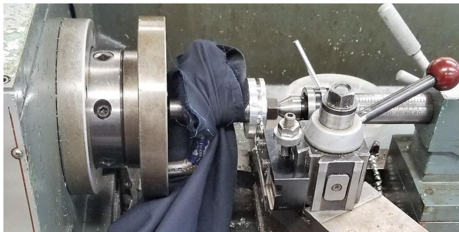
Figure 3: Student's Lab Coat Caught on a Lathe Dog
