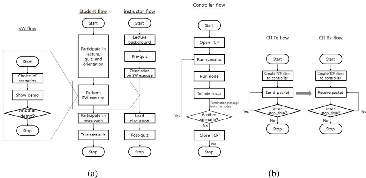
Figure 2 (a) Structure of a typical tutorial, with flowcharts showing instructor, student, and software actions. (b) Structure of a hands-on exercise showing flowcharts for the experiment controller (part of CRTS) as well as two cognitive radios (CRs) that are part of the exercise.
