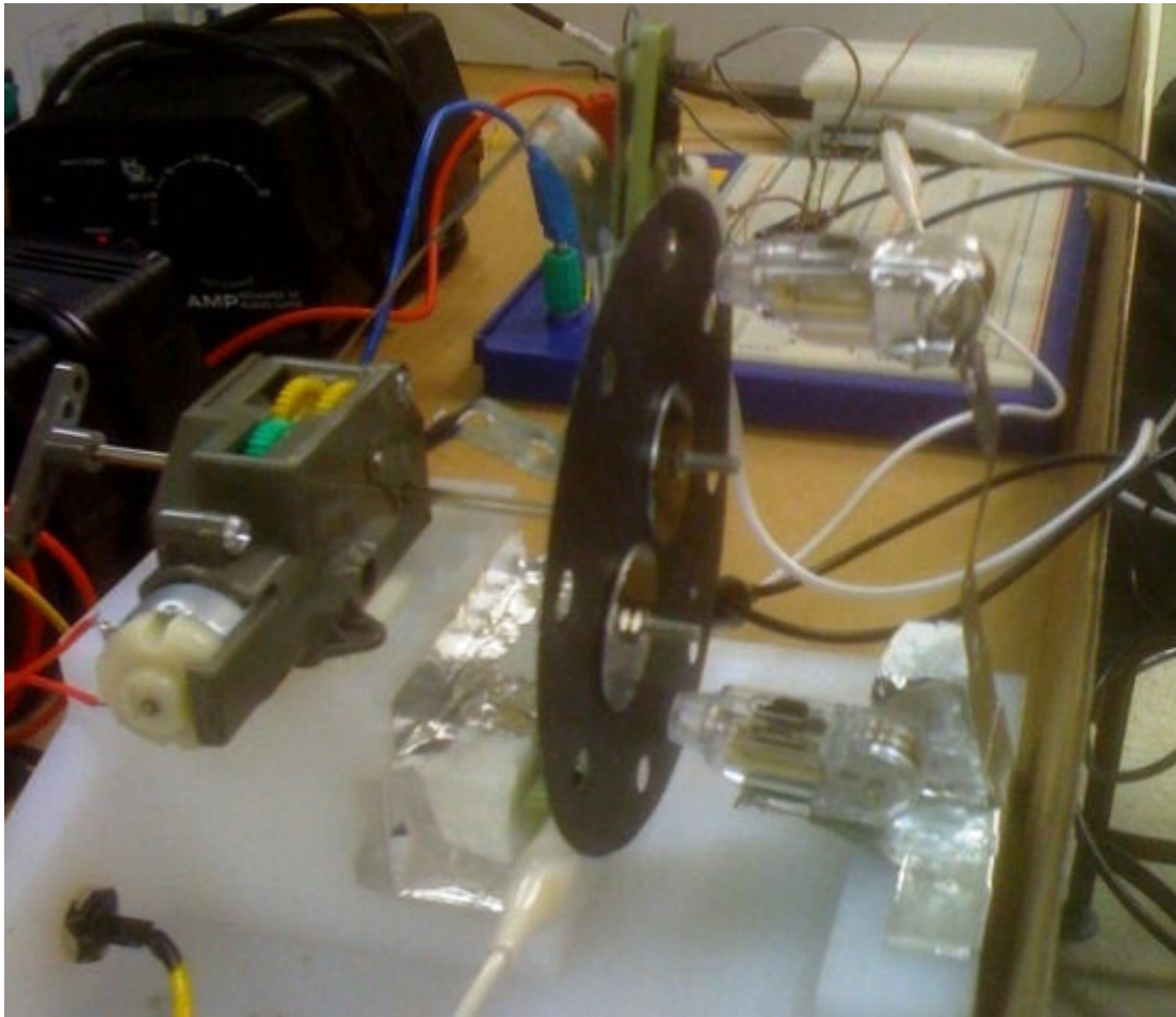
Figure 6: Encoder/Tachometer Lab Project
