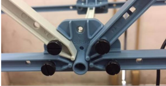
Fig. 3 Gusset Plate in the Experiment
