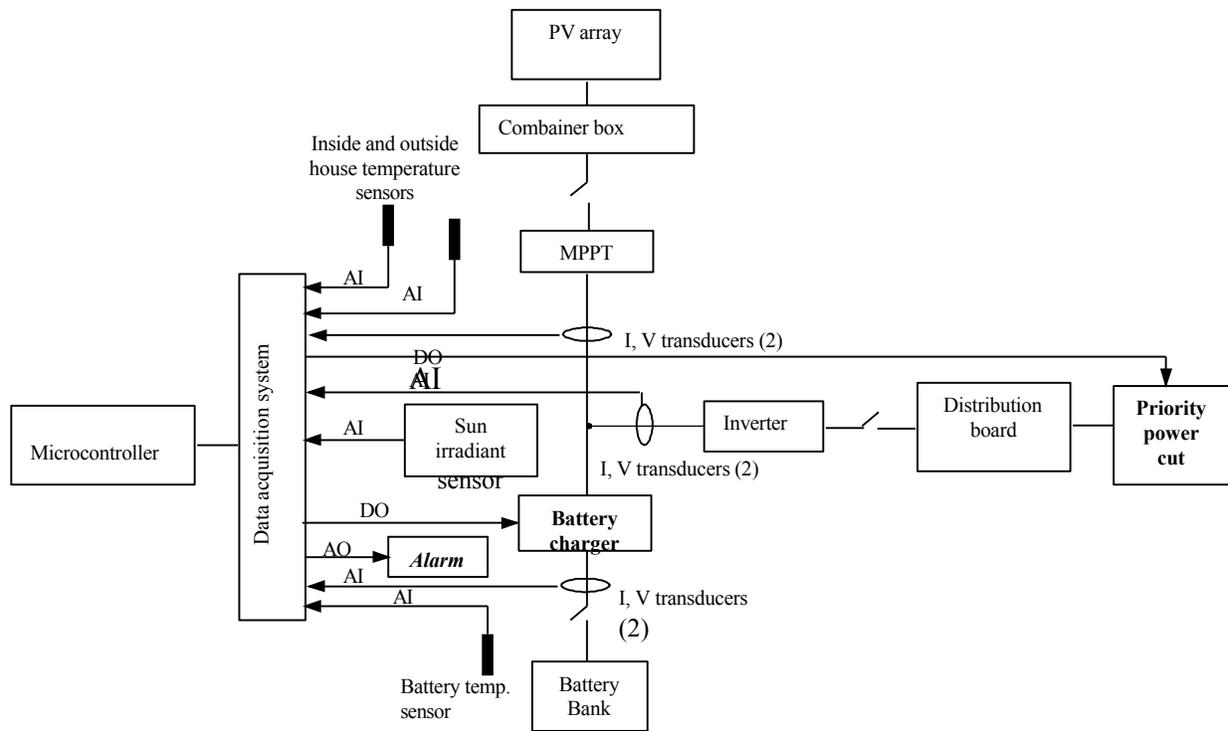
**Fig. 2** Block diagram of monitoring/control of a stand-alone solar house
