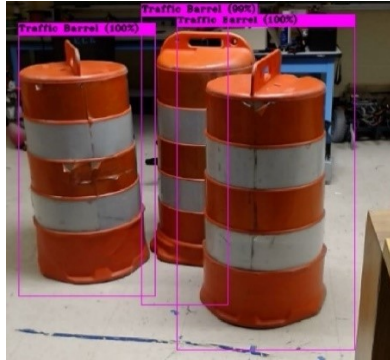
Figure 8: Classification of overlapping traffic barrels
