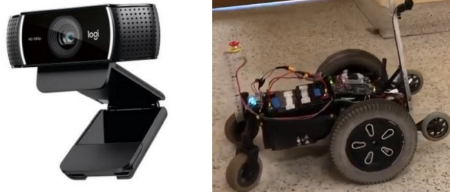
Figure 3: (a) Camera (b) Camera mounted on the IGV
