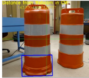
Figure 10: Detection and Distance Estimation by the Python program
