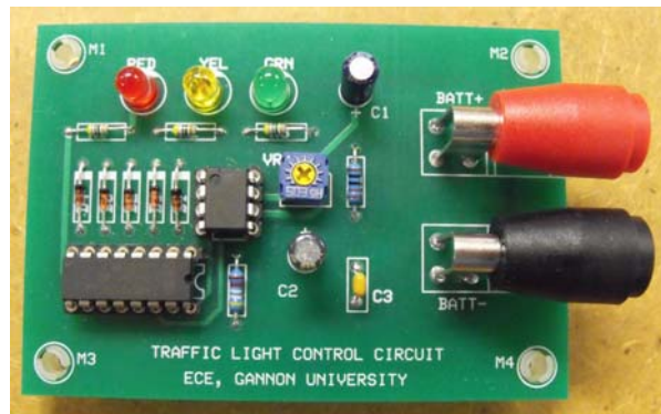
(b) PCB-based protoboard
