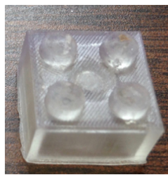
SLA Brick: Photo and Digital Image of Side Surface Showing Layers
