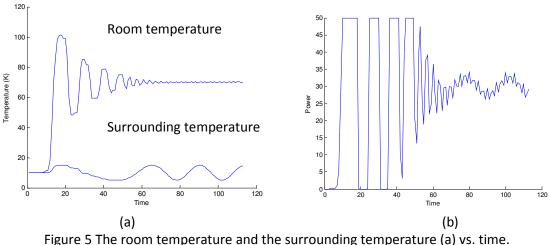
Figure 5 The room temperature and the surrounding temperature (a) vs. time. The power supplied from fuel cell system (b) vs. time.
