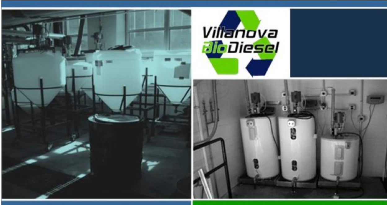
Figure 8: Nalgene hoppers used for biodiesel separation from glycerin by-product
