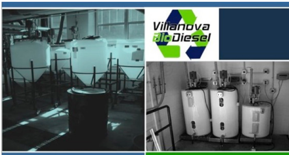
Figure 16: Nalgene hoppers used for biodiesel separation from glycerin by-product.
