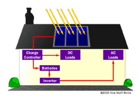
Figure 3, Typical Residential Solar Electric System
