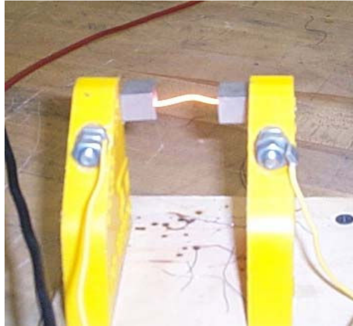
Figure 5 - Heated Wire before Break
