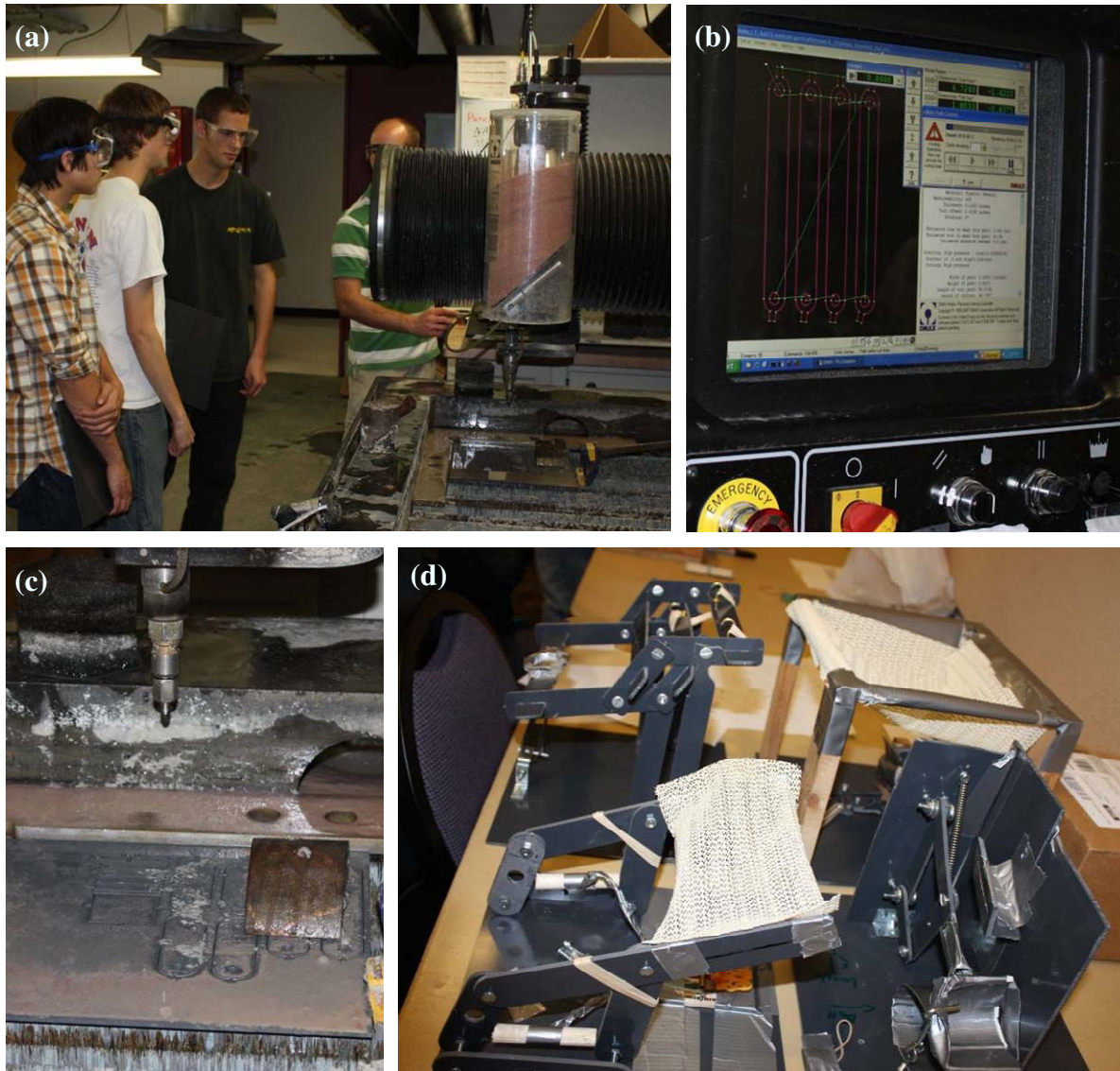
Figure 2. (a) ME 1000 students manufacturing fourbars on the waterjet cutter in the ME machine shop. (b) The students' CAD drawing on the waterjet computer. (c) The waterjet nozzle above several cut fourbars. (d) A set of "volleybots" with fourbars.
