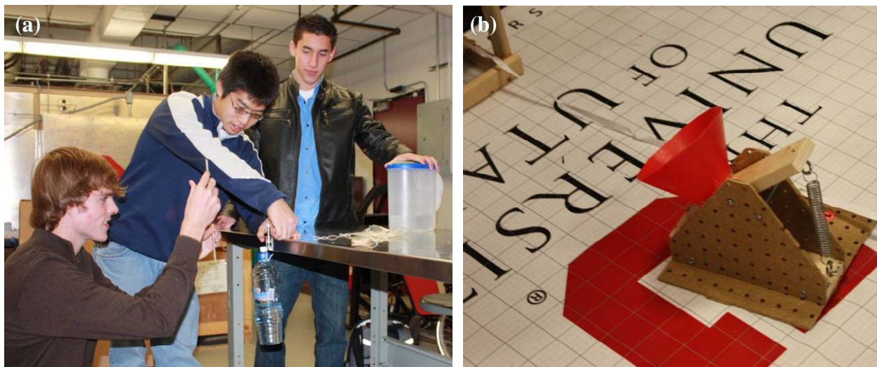
Figure 4. (a) ME 1000 students performing displacement vs. force measurements on springs. (b) A “volleybot” utilizing a spring for its mechanical power source.
