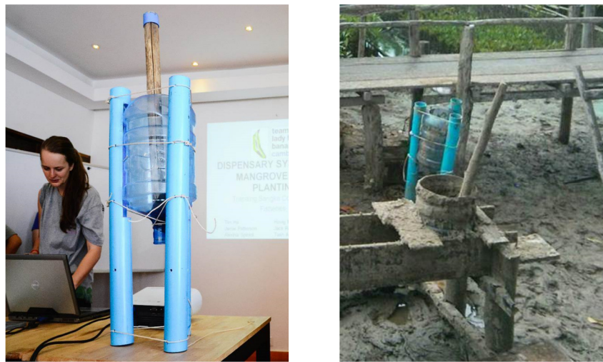
Figure 2: Mud bag filler, with the prototype concept developed by students on the left and the design as implemented by the partner on the right, with the prototype in the background.
