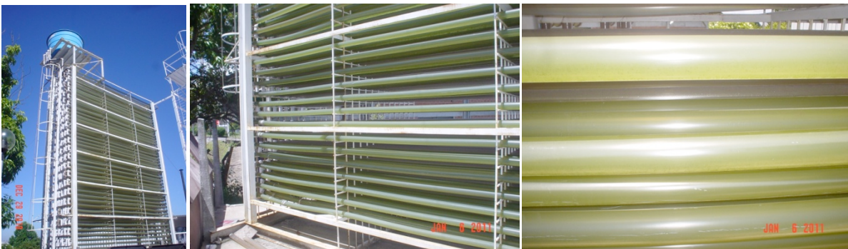
Figure 1. Microalgae growth in compact photobioreactor (5 m × 2 m × 8 m) at the Brazilian university
