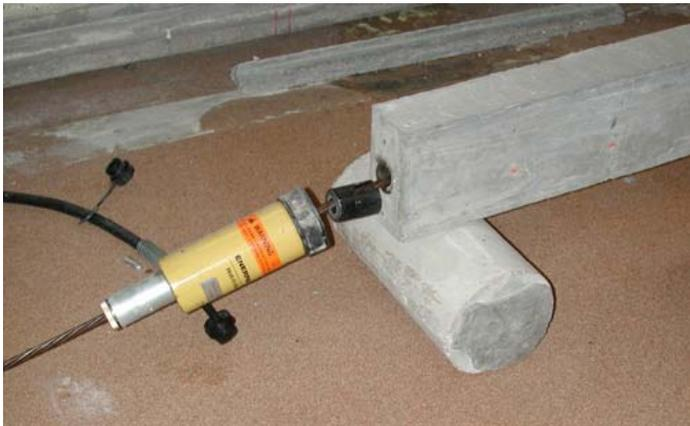
Figure 7 - Two span continuous beam used to teach post-tensioning techniques
