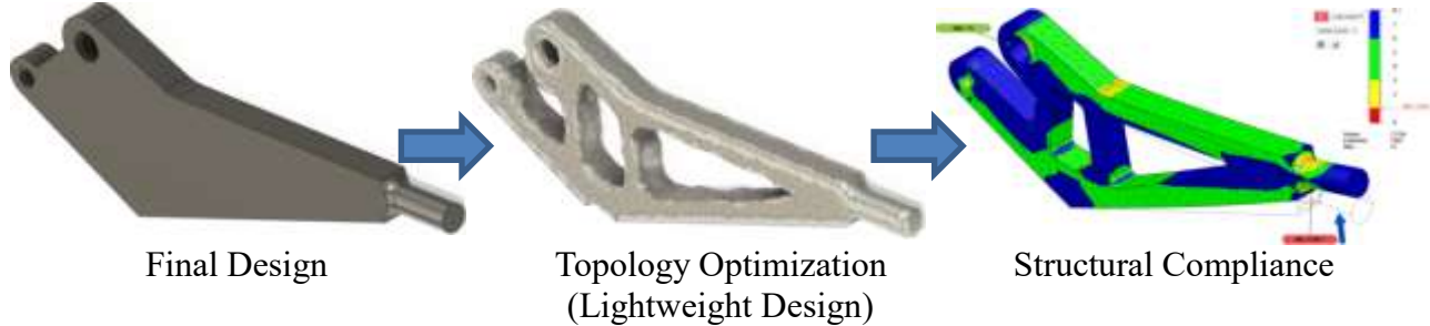
Figure 2. A sample design project demonstrating shape (topology) optimization in Computer Aided Engineering
