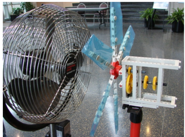
Figure 12. A student-built turbine showing the turbine blades attached to a small-to-large gear ratio that is attached to the spinning axle.
