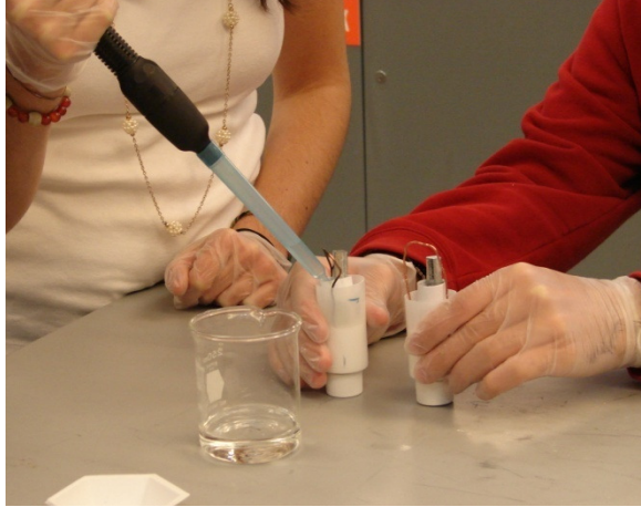
Figure 5. Students initiate the chemical reaction in the battery cell that will conduct a useful current that will power a motor attached to a spinning axle and weight system.
