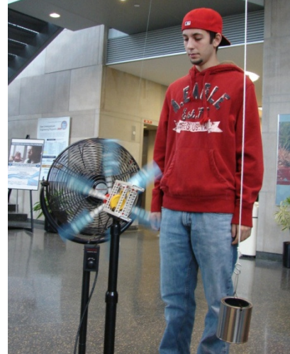
Figure 4. A mechanical fan creates wind that powers a turbine system connected to a spinning axle via a system of gear ratios. A string attached to the weight is connected to the axle by a pulley.
