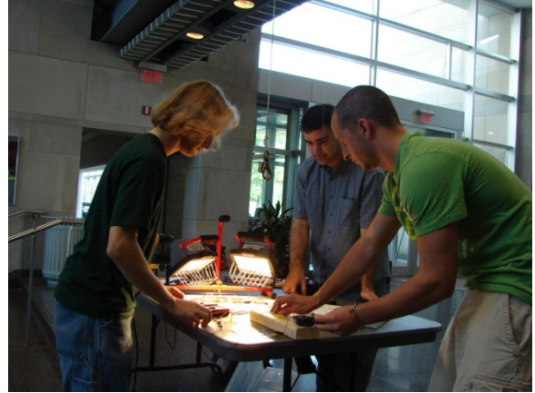
Figure 7. Students attach their chosen PV array to the motor and pulley system.
