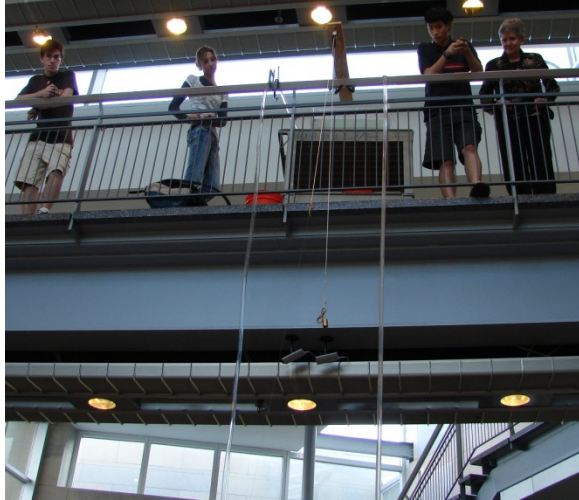
Figure 3. For the hydropower experiment, a storage tank of water is placed on the second story walkway and the water is fed to the turbines on the first floor via a plastic tube.
