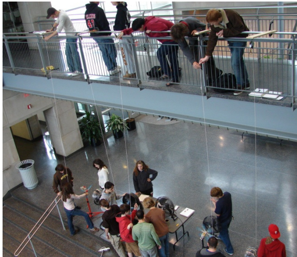
Figure 1. Pulley system set up at a measurable distance above the testing station. The weights are tied to a string that is run through the pulley and attached to a spinning axle.
