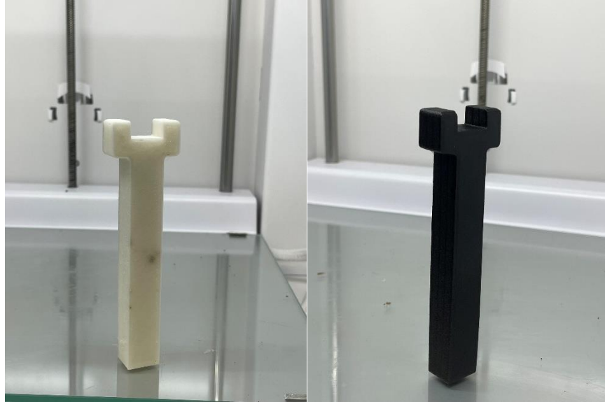
Figure 8 – Functional parts for high-temperature applications (140°C - 150°C) printed in NylonG PA-GF (left) and NylonX PA-CF (right) [12], [13], [15].
