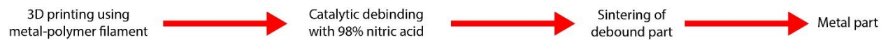
Figure 2 – Printing, debinding, and sintering process chart for BASF Forward AM 17-4 PH SS filament [9].
