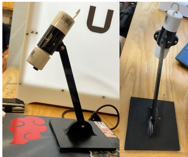
Figure 1 – A 3D-printed holder for a filament heater. This holder was printed using Ultimaker PLA. 3D printing can be used for many such applications for functional parts [6].
