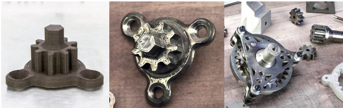
Figure 9 – Gear printed with BASF Forward AM 17-4 PH Stainless Steel Filament (left). Gear in stainless steel after sintering (middle). The gear inside the assembly is fully made using BASF's SS Filament (right). [7], [9], [18]. Image from www.matterhackers.com
